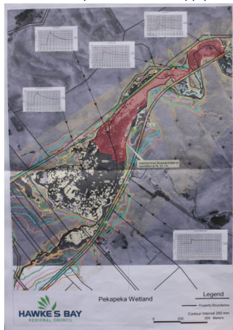
Fig 4: Modelling identified the extent of inundation with the appropriate levels.
