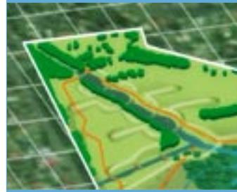
**Above: the system of channels and forebays and bunds. showing how it deals with flooding by distributing this bund by bund. Below: the overall treatment process including the perimeter channel and the rest of the reserve.**
